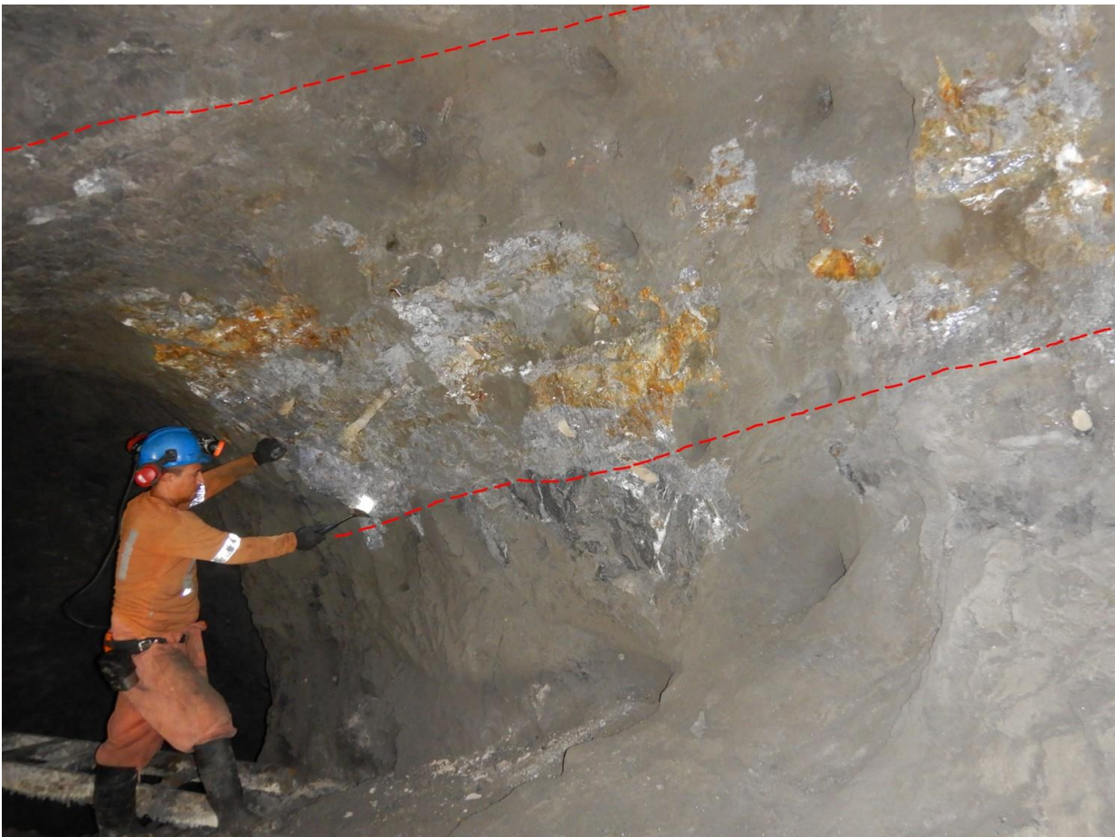
Figure 4. Tres Amigos massive sulphide exposed on Level 5 prior to first mining cut. Channel sampling returned 2m at 19.1% Zn+Pb from this face.
