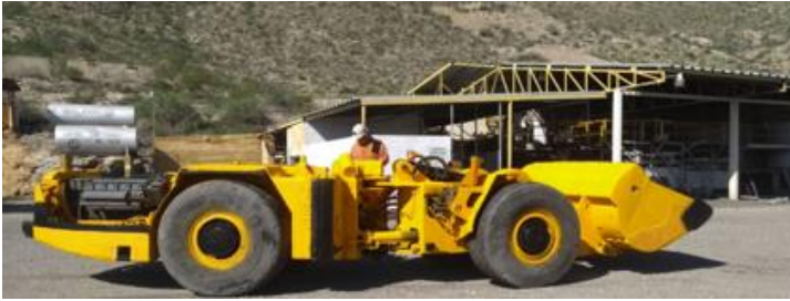
Figure 2. CZL's 5-yard Scooptram (ST#5) on site
