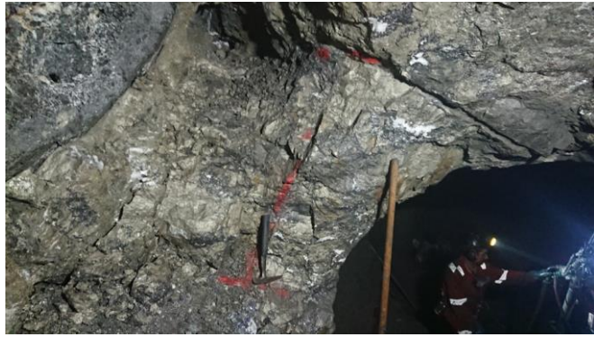
Figure 4. Tres Amigos high grade ore exposed in stope 1000. Note the hanging wall contact in the top left corner of plate with low grade running >5% Zinc.
