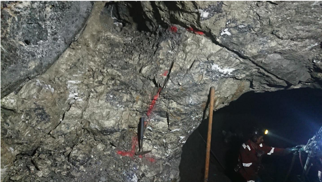
Tres Amigos high grade ore exposed in stope 1000. Note the hanging wall contact in the top left corner of plate with low grade running >5% Zinc. Miner in the bottom right corner shown drilling out the next round.
