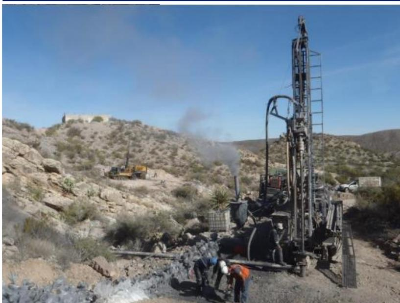
Figure 1. RC and diamond (background) rigs on surface at Plomosas
