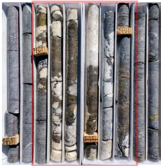
Figure 3. Massive sulphide mineralisation in the Cuesta shales intersected in LV5054 drill hole between 149.45 to 152.55 metres (3.1m). This 3.10m intercept is the deepest intersected by CZL to date and assayed at 18.8% Zn, 1.25% Pb and 13.22 g/t Ag.
