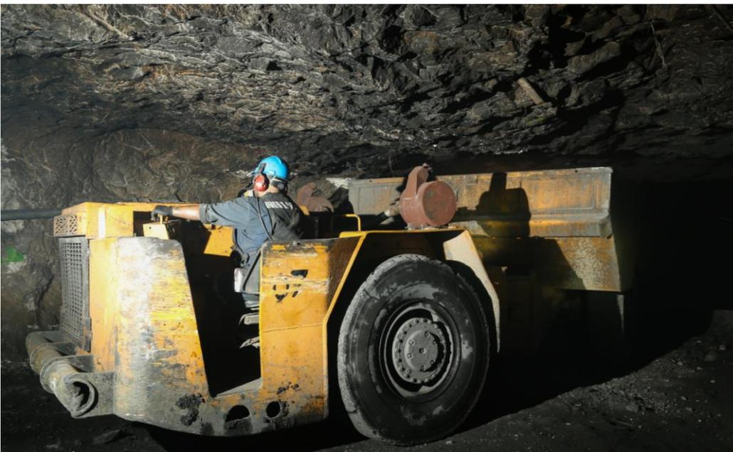
*Moving broken ore within the stopes*
