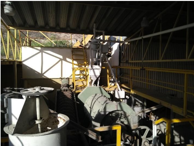
Photo 1: The reagent mixing area in the foreground, mill to the right and the white fine ore bin in the
