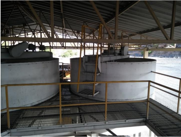
Photo 5: The 3m 3 lead concentrate thickener
