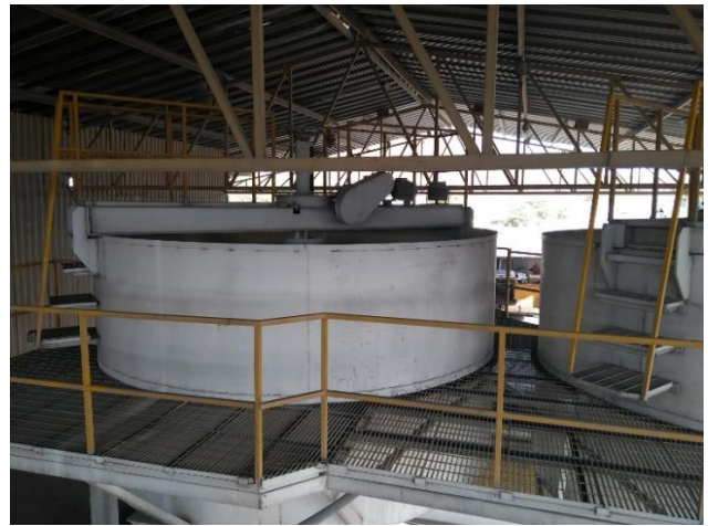
Photo 6: The 5m 3 zinc concentrate thickener
