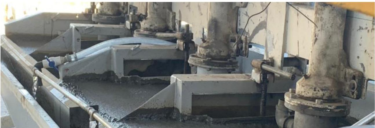
*Picture 2: Flotation cells.*
